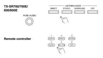
**PURE AUDIO (PURE A) (TX-SR700/700E only):** Changes the listening mode for the signal type that is currently being input from the selected input source to the Pure Audio listening mode. If pressed, the corresponding setting in the "Input Setup" menu for the selected input source is also changed (see page 54).
